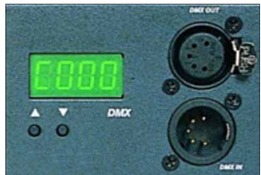
example control panel of a DMX dimmer
