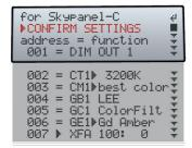
set-up Skypanel-C # to "Mode 2", 8-bit, set DMX address 001
