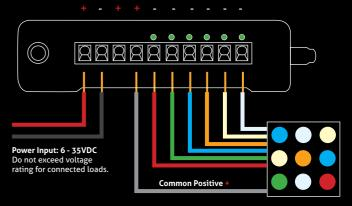
The illustration on the previous page shows an RGBATD (T is tungsten or warm white, D is daylight or cool white) color mixing LED device. There are 7 wires: a grey wire for the 12V common positive (+), and six colored wires, red/green/blue/amber/tungsten/daylight, for the six unique negative loads. The color of the common positive may vary, it is not always grey.
